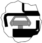
Fig. 62: C-shaped rail and guide rollers
